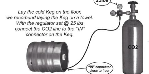
NOTE: The "IN" connector on the bottom close to the floor.
