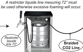
IMPORTANT: To eliminate the back flow of beer from the Keg to the CO2 regulator. Remove CO2 from Keg by quickly pulling on the pressure release valve. Set the regulator to 12 - 13 lbs on the CO2 tank. Connect CO2 line to the "IN" connector and the liquid line to the "OUT" connector on the Keg. Pull tap and discard the first glass, the second glass should have a 1" thick head. Enjoy!
